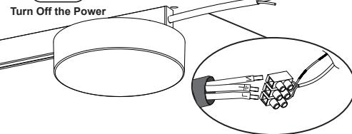
Remove the wire from one end of the power supply
