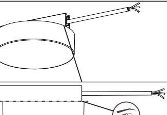
After installing the power supply, observe whether the power supply is firm and completely flat on the magnetic track with a "click" sound feedback
