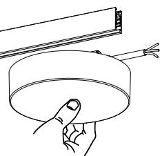
Align with the track and insert vertically
